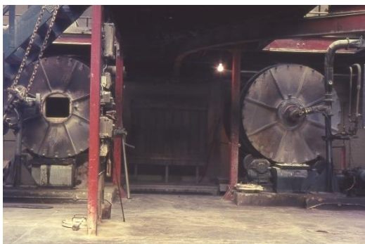
Furnace left, with burner swung clear.
