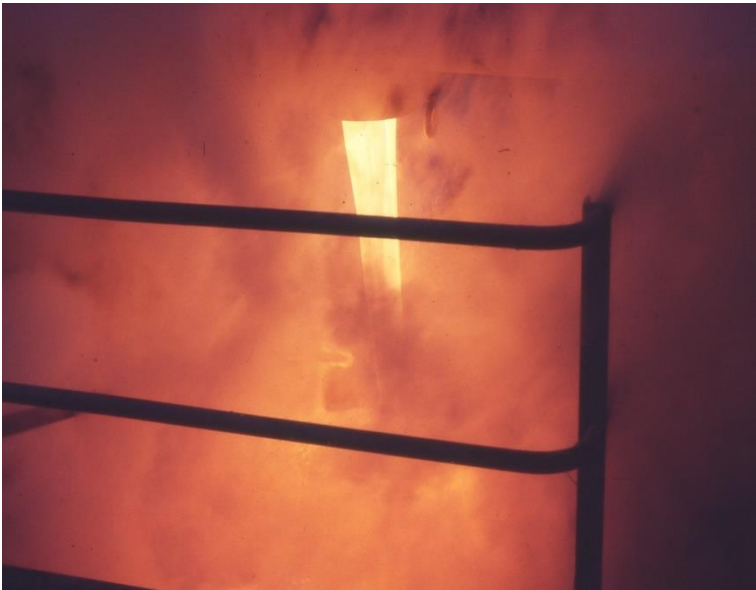
Melt pouring through the vast amount of steam generated.
