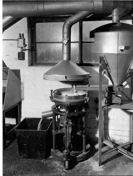
Photo right, dry colour sieving unit.
