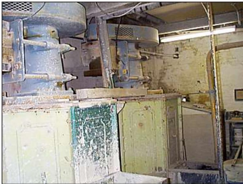
The blunger washes the clay and converts it to slip.
