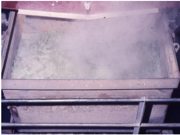
Steel basket being lifted from the water-bath to allow the water to drain.
