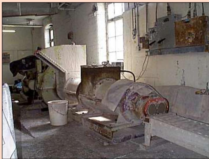
The pug mill at Burgess and Leigh did away with the need for the air to be removed from the clay by 'throwing' it.
