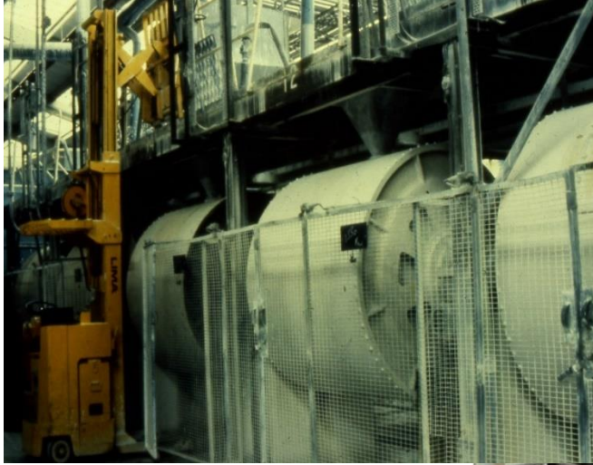
Modern Ball Mills – loading platform above.
