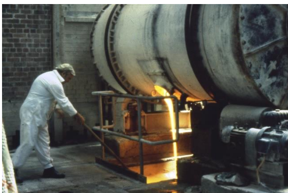
Two more photo-images of frit furnaces during the pouring operation.
