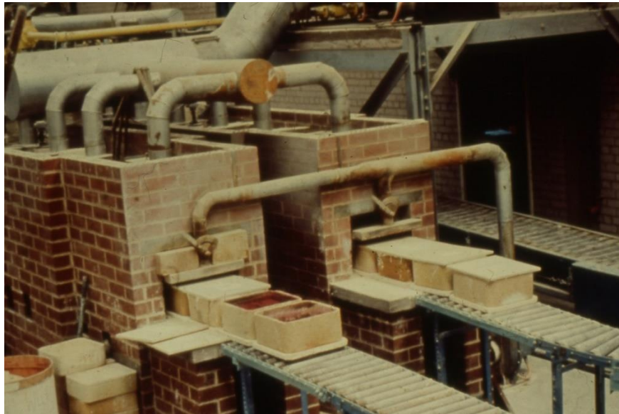
Dual tunnel kiln – colour saggars emerging.
