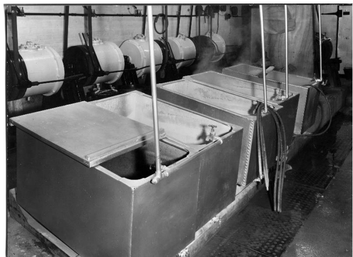
Milling colours, above and right, washing tanks (after washing the colour solids settle and surface water is siphoned away to drain) - photos c.1950's.
