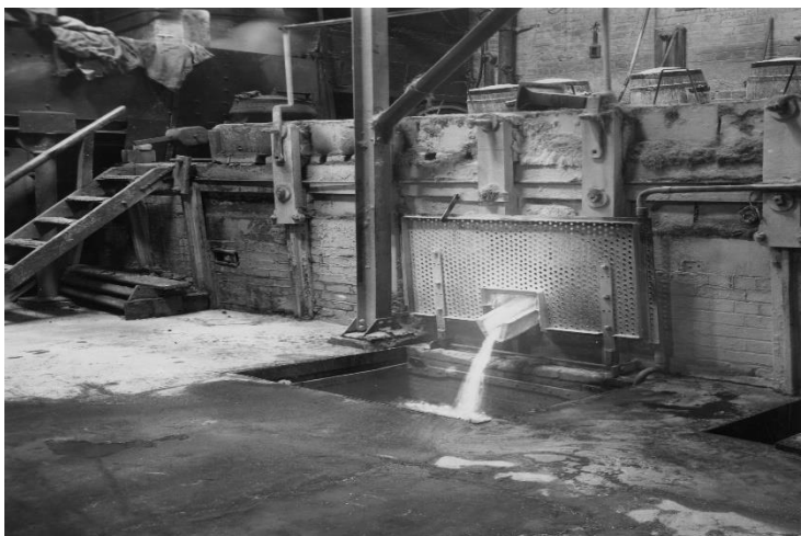
Molten frit discharging from a reverberatory furnace into the water-bath.
