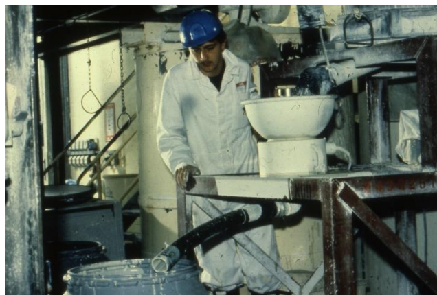
Glaze passing through electro-magnet (c.1980's)
