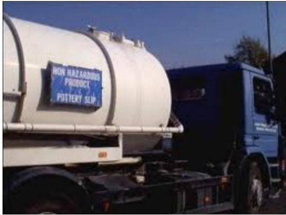
Steel tank (pressure delivery)
