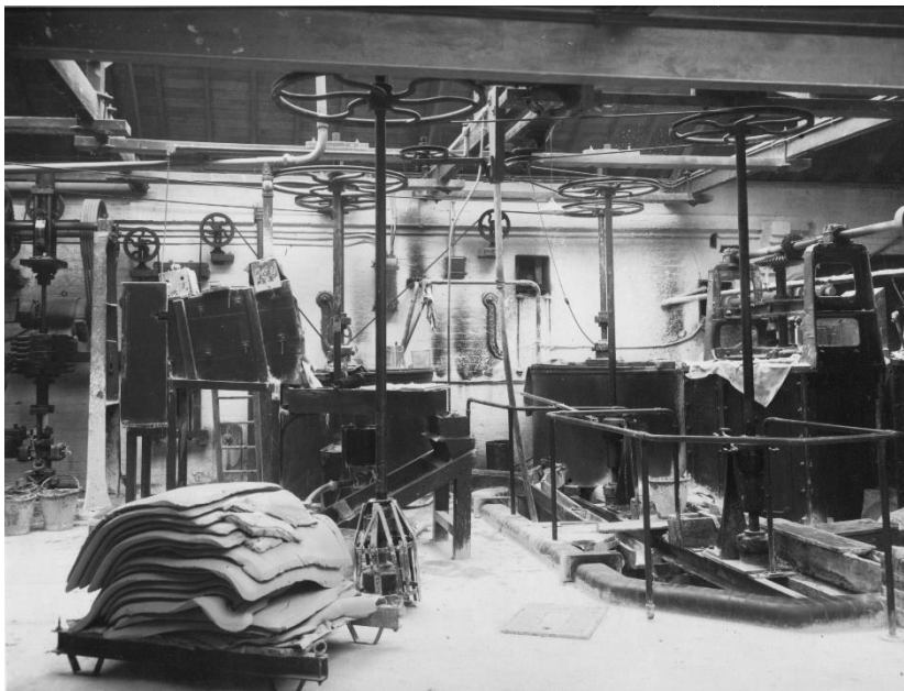
Sliphouse (c.1940's). Mixing arks below ground to the right foreground. Plastic clay press-cakes on the pallet. Note the amount of belt-drive machinery.
