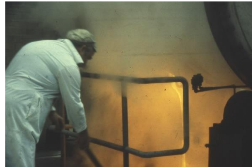
Operative commencing a pour.
