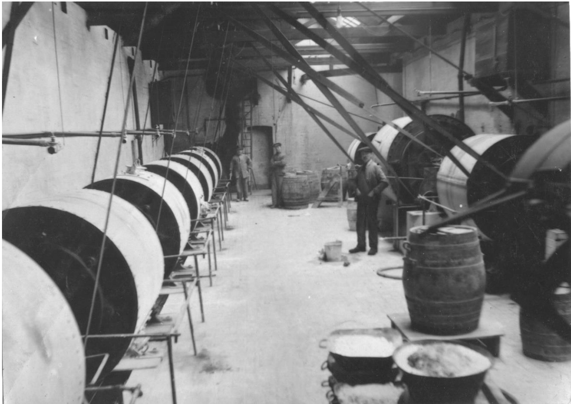
Picture shows belt driven ball mills (c.1950). In foreground weighed glaze material in troughs ready to load into a mill.
